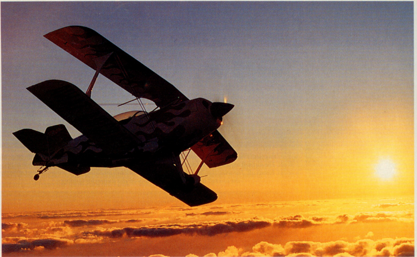
The new Pitts, shown here at the start of a snappy breakaway maneuver, can now roll at 300 degrees per second, an increase of at least 60 degrees. Testing was not complete when these photos were taken. Certification is expected this month.
