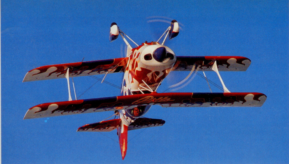
Against this clear blue sky over the Florida Keys (above), the Pitts S-2C is upside down, a favorite mode of flight. The aircraft requires only a quarter inch of movement of the trim lever in the rear cockpit to fly inverted, hands off. The wing tips have been squared off (bottom), providing more wing area and allowing the aircraft to float more than the S-2B did during the landing.
